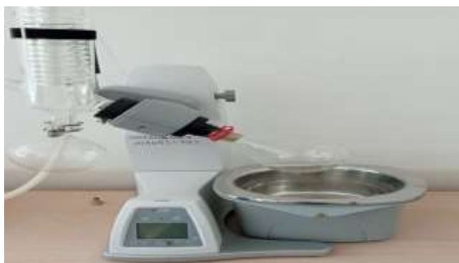
Figure 4. Rotary Evaporator Extraction Process
