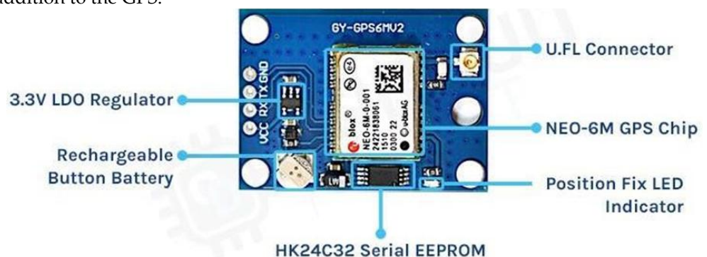
Figure 5. Structure of GPS NEO 6M
