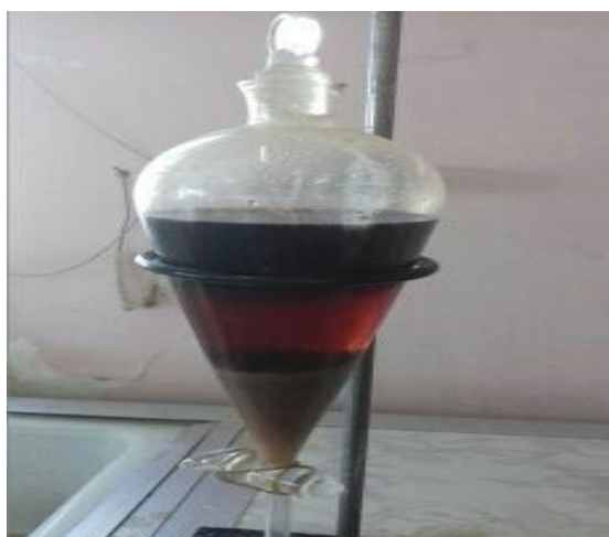
Figure 1. Separation funnel instrument for alkaloid.
