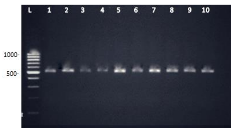
Figure 8. Gel electrophoresis of PCR CTX-M gene (550 bp.) of P. aeruginosa Lane L. DNA marker (3000 bp). 1-10 result positive
