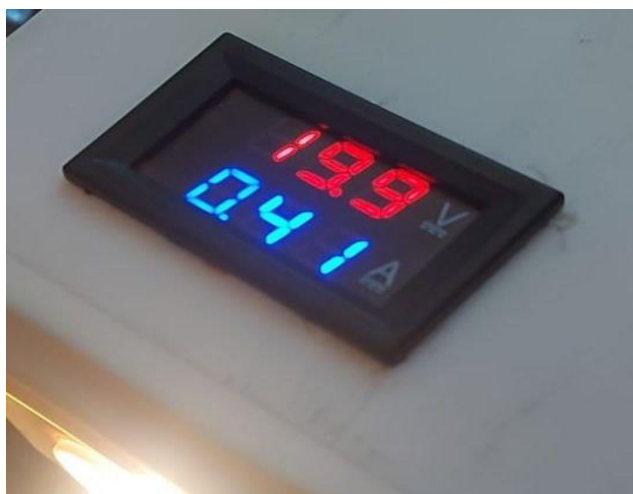
Figure 9. Voltage panel meter showing 19.9V and 41mA
