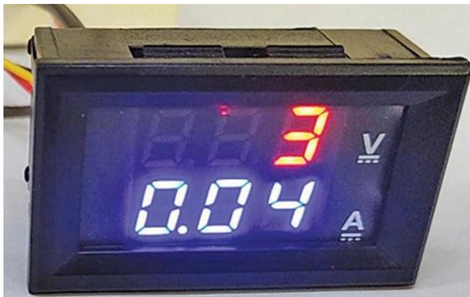
Figure 8. Voltage panel meter showing 3V and 40mA
