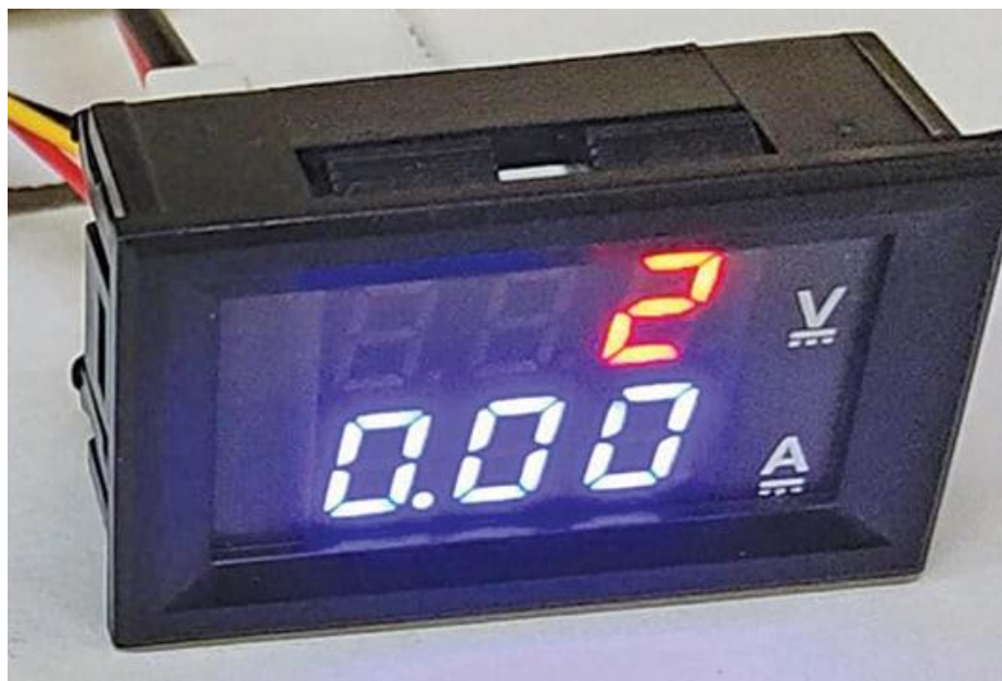
Figure 7. Voltage panel meter showing 2V and 0 mA
